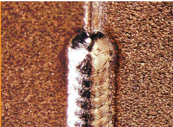
Fig. 1 Top surface of butt welded titanium
