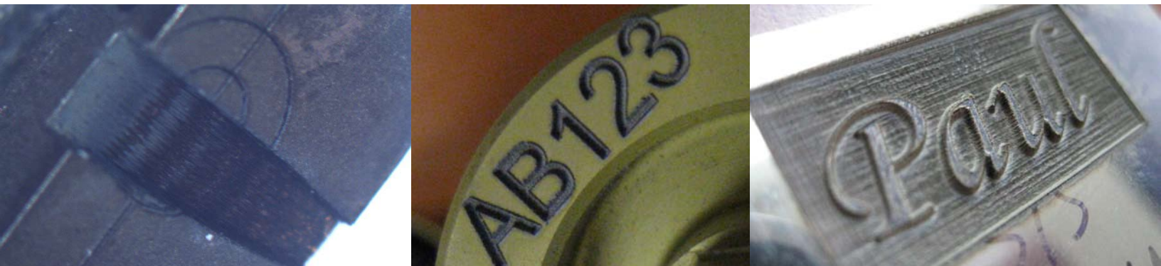
Deep engraving in Inconel (left), anodized AL (middle) and silver (right)
